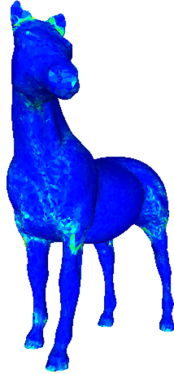
Figure 2: The absolute differences in SDF value between each face and its neighborhood, coded from blue where close to zero to red where maximum, shows that the function has very small variations on most of the surface
