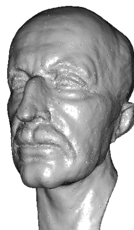
Figure 1: Max Planck point cloud rendered at 4.5 fps on an AMD HD4850 GPU. The viewport size is 640 by 480. The model consists of 96208 surfels.
